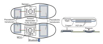
Fig. 3. Components on two shoes.
