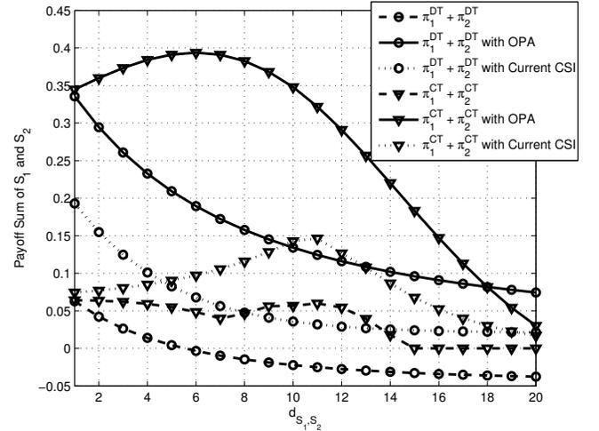
Fig. 6. Numerical results for the payoff sum of  $S_1$  and  $S_2$  in SSS based CR networks with multi-hop relaying
